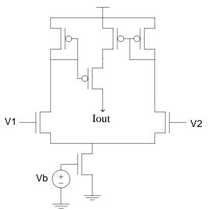
2. Solve for  $I_{out}$  as a function of the difference of the two input voltages  $(V_1 - V_2)$  for below threshold CMOS operation. As usual, first, assume  $\kappa = 1$  and derive your answer. Then assume  $\kappa$  is the same for all transistors but not equal to one and derive your answer. Simplify your expressions as much as possible. Show all of your work and explicitly state all assumptions, e.g. which transistors are in saturation, subthreshold operation, matching of devices, etc.
