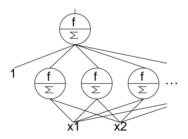
In doing an assignment, a student forgot to include the bias at the input layer. The student did remember to include the bias for the second layer– the resulting architecture is shown in the above figure. An arbitrary number of hidden units may be added but no additional hidden layers can be included. Assume the sigmoid activation function of the neural network to be:
