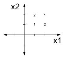
Assuming that four data points are given as shown above, can this problem be solved using this single hidden-layer architecture with no bias in the input layer? Justify why or why not. If possible, provide all of the necessary weight values for the architecture with the minimum number of hidden units. The final output of your neural network should be +1 for class 1 and -1 for class 2.
